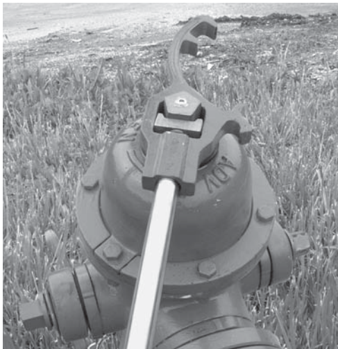
Wide bearing surface on wedge nut grips and retains operating nuts better than conventional threaded handles.
