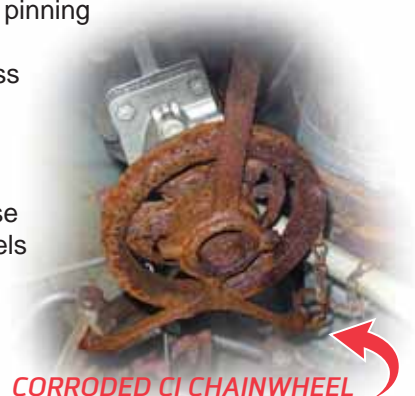
CORRODED CI CHAINWHEEL shows advantage of stainless
