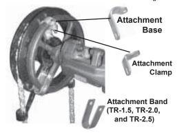
Use Attachment Bases with Clamps (a Band is used in place of one Clamp Assembly on smaller sizes) to secure the Chainwheel to the valve handwheel as shown above. Slots in Chainwheel allow adjustment for range of handwheel diameters; slots in Base and Clamp allow adjustment for various handwheel rim diameters.
