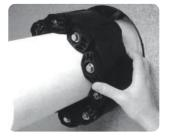
Wrap the belt around the pipe and connect the first and last links together.
