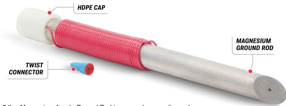
The 1.5 lbs. Magnesium Anode Ground Rod is an anode grounding rod designed for seamless integration into tracer wire systems to complete the electrical circuit necessary for enhanced signal detection. The anode ground rod has a diameter of 1.31 inches and a length of 18.5 inches, making it compact yet effective for its intended application. Its design ensures secure placement within backfill environments, optimizing electrical conductivity and signal transmission.
