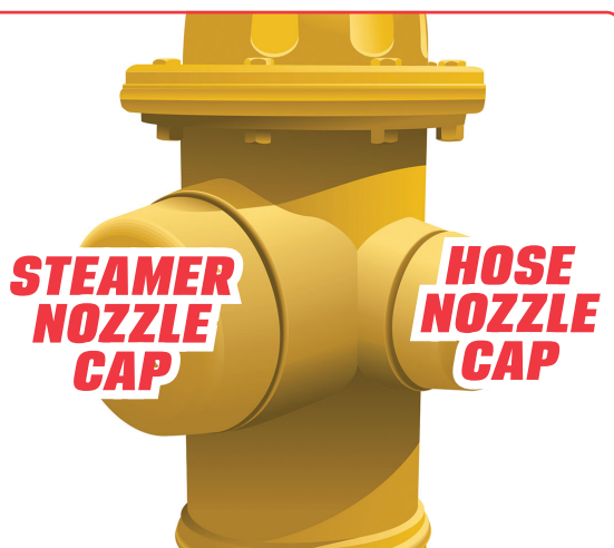
ILLUSTRATION SHOWING THE DIFFERENCE BETWEEN HOSE AND STEAMER NOZZLE CAPS.
