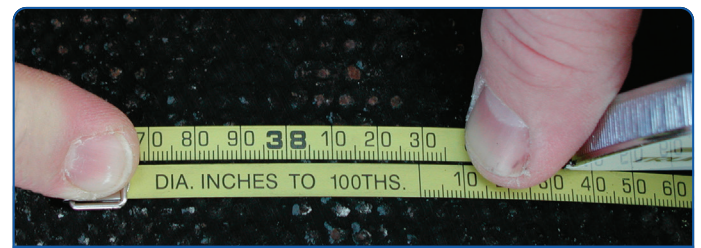
TRUMBULL'S 10 FOOT TAPES CAN MEASURE THE OUTSIDE DIAMETER OF 36" DUCTILE PIPE (38.30" O.D.)
