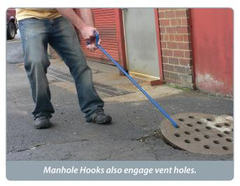
Trumbull Manhole Cover Hooks are made of 5/8" hexagonal steel. The 1/2" point engages the lid of the manhole cover.
