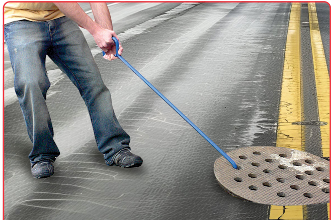
MANHOLE HOOKS ALSO ENGAGE VENT HOLES.
