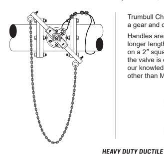
Trumbull Chain Levers save the unnecessary expense of adding a gear and chainwheel to valves that don't require a gear to operate.
