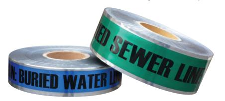
Tape consists of an aluminum core encased in plastic. Stocked in 1,000 foot rolls in standard industry colors. For installations 30" or shallower, 2" wide tape should be used. For deeper installations, 3" tape should be used. Use electronic pipe/cable locators for best results (as opposed to valve box or metal locators).
