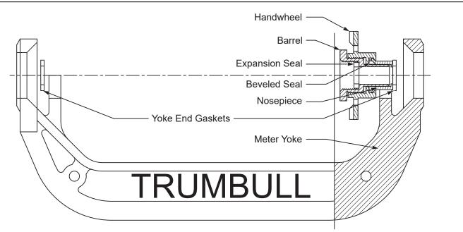
Barrel and Nosepiece are in contact with potable water and will conform to UNS C89833. They will be marked, "NL", and are certified by UL for compliance with NSF/ANSI 61 and NSF/ANSI 372, per the U.S. Safe Drinking Water Act. EPDM and fiber seals meet NSF/ANSI 61.
