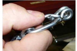
First tail trimmed from first loop.
