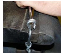
3.) Pry open the two trimmed loops, to insert the new chain link.
