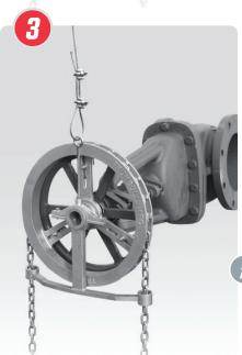
Loop cable through eyebolt leaving about 6" excess.
