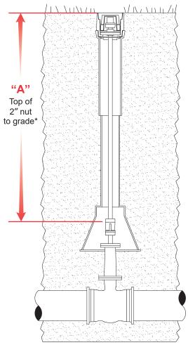
\* The dimension from top of 2" valve nut to grade is used to determine Extension Stem length, per ordering instructions on page F-1.
