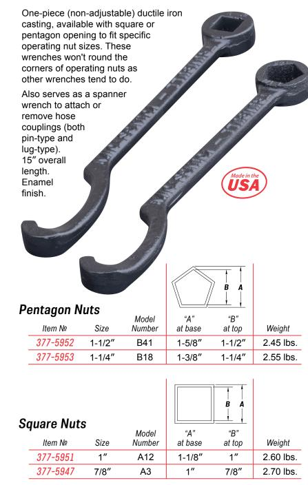
Other sizes and shapes available upon special request. Please give dimensions measuring "point to flat" for pentagon nuts or across center from "flat to flat" for square and hexagon nuts.
