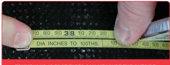
TRUMBULL'S 10 FOOT TAPES CAN MEASURE THE OUTSIDE DIAMETER OF 36" DUCTILE PIPE (38.30" O.D.)
