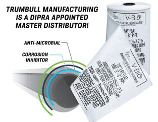
V-Bio<sup>®</sup> Polvethylene is a minimum 8-Mil co-extruded linear low-density polyethylene film infused with additives that enhance ductile iron pipe's ability to provide the long service life that is the benchmark of ductile iron pipe. Meets all requirements of the American National Standards Institute and the American Water Works Association (ANSI/AWWA C105/A21.5) standard for polyethylene encasement.
