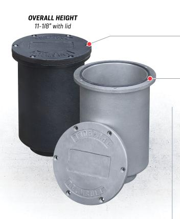
Trumbull Sealed Floor Boxes are ideal to prevent fluids and vapors from penetrating the floor slab from either direction. Top side is sealed by a Buna-N O-ring, and bottom side can be sealed by use of optional packing gland. Overall length is 11-1/8", but the underside is tapped to accept 2-1/2" NPT steel pipe nipples for floors thicker than 11".
