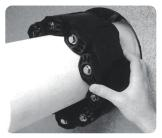
Wrap the belt around the pipe and connect the first and last links together.
