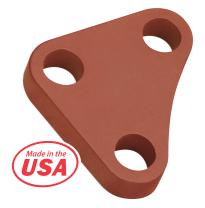
Also known in the field as "Thrust Plates", "Harness Lugs" or "Gusset Plates". They are installed on the back sides of ANSI Class 125 B16.1 and Class 150 B16.5 flanges to allow tie rods to span across an unrestrained piping component.
