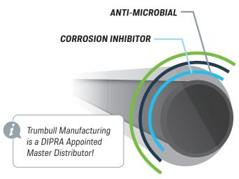
V-Bio® Polyethylene is a minimum 8-Mil co-extruded linear low-density polyethylene film infused with additives that enhance ductile iron pipe's ability to provide the long service life that is the benchmark of ductile iron pipe. Meets all requirements of the American National Standards Institute and the American Water Works Association (ANSI/AWWA C105/A21.5) standard for polyethylene encasement.
